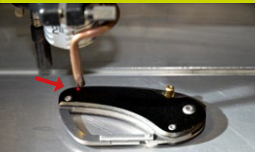
Acquisition of the shape to be engraved using the Point & Shoot red light pointer
