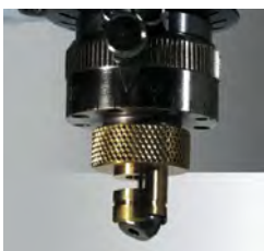
Steel swivel nose Ø 2.5 mm (.1") Ref. 22464
